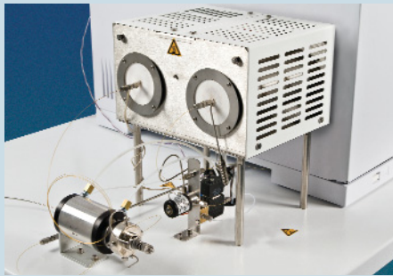
Nu GC-IRMS interface attached to the Agilent 7890 GC
