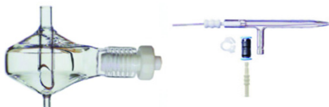
Figure 1: Wet plasma sample introduction system consisting of baffled cyclonic spray chamber and microconcentric nebuliser, both manufactured by Glass Expansion.
